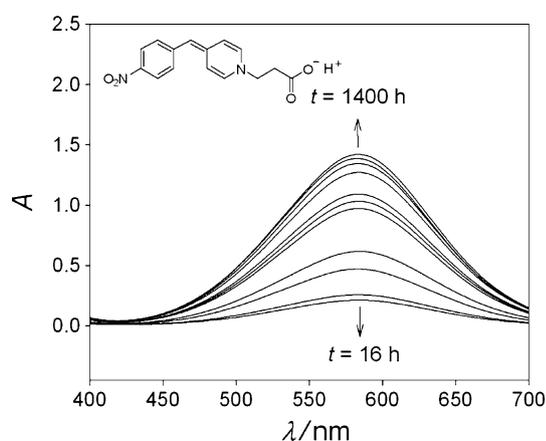
**Fig. 1** Formation of the NBP–AA adduct over time. Variation in absorbance in the 16–1,400 h range in 7:3 water/dioxane medium.  $[AA]_0 = 0.1$  M;  $[NBP]_0 = 2.5 \times 10^{-4}$  M;  $\theta = 35$  °C; pH 3.5
