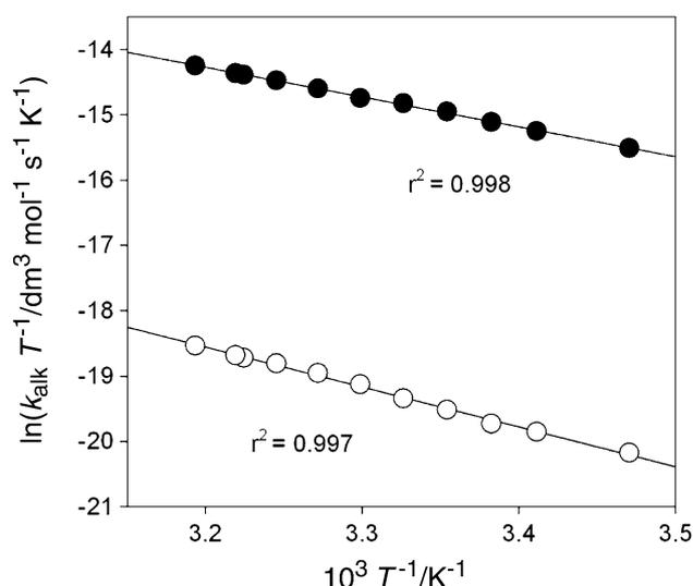
**Fig. 3** Eyring plots for NBP alkylation reactions by AN (filled circle) and AA (open circle) in 7:3 water/dioxane medium
